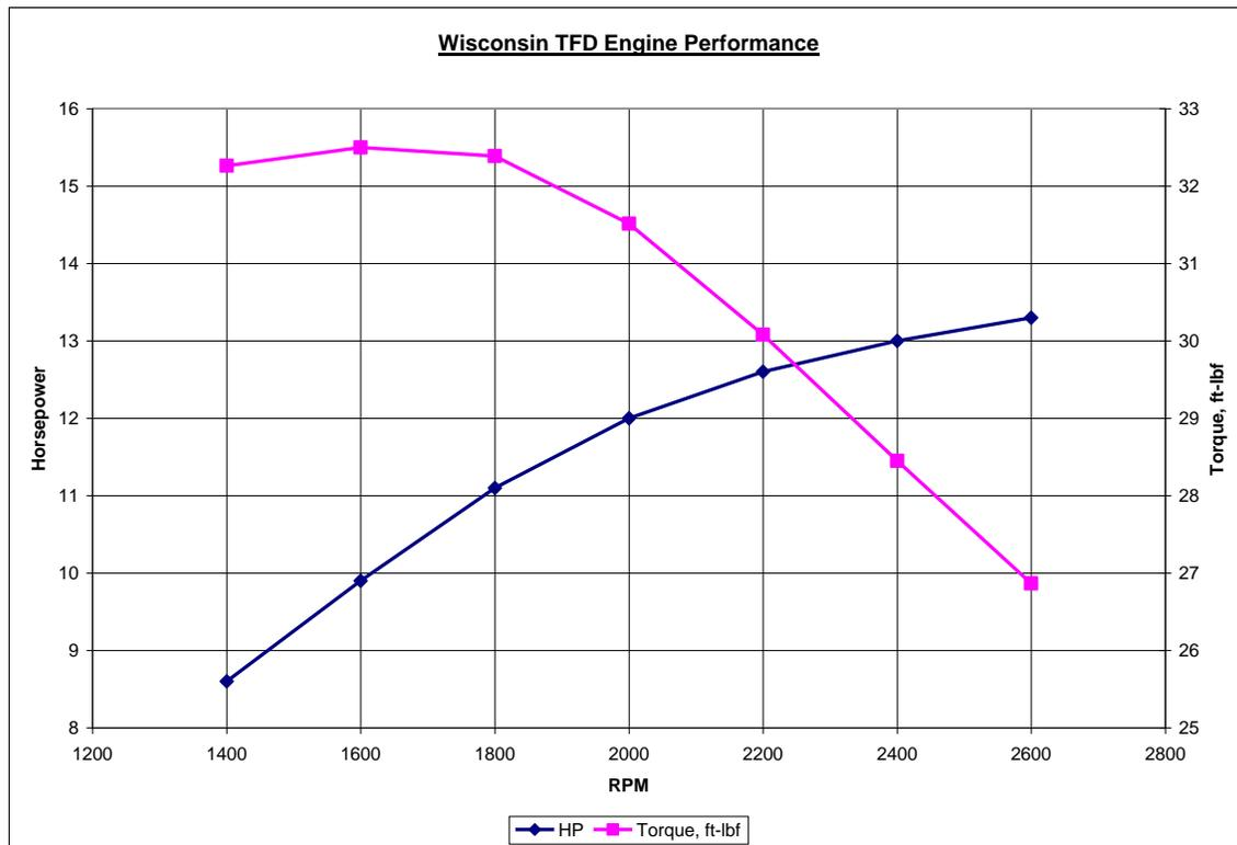
Note that the horsepower is still climbing at the 2600 rpm rated speed and the torque is still respectable at 27 ft-lbf. What is really impressive is the torque values at a relatively low 1600 rpm – a whopping 32.5 ft-lbf!
