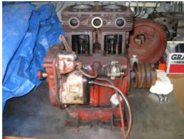
Pistons were so loose in their bores that they would rock from side-to-side as the engine was rotated over TDC. The cylinder walls were glazed to a dull mirror finish. The intake valves were so worn on their seating surface that they weren't worth regrinding. The exhaust valves however, were in perfect shape!
