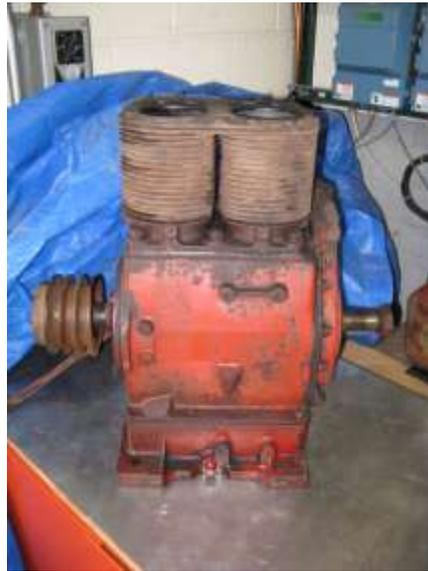
Removing the valve spring covers proved that this engine had been running hot – black, carbonized oil was present.
