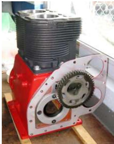
New, .010 over pistons and ring sets were purchased and a good friend and Wisconsin engine expert, Mr. Bill Zubella, kindly donated a pair of brand-new connecting rods to my project. The crankshaft was in perfect condition – the large Timken roller main bearings were in like-new shape. The crankpins were polished with a Scotch-Brite pad to a mirror-like finish.
