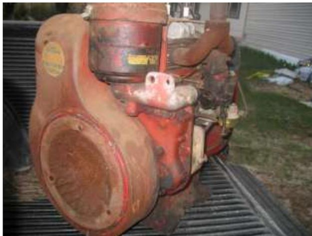
With gasoline supplied from a remote tank, the engine started right up using the handwheel starter. Gas dripped from the carburetor and some light blue smoke was visible in the exhaust, but it ran and I was encouraged. My plan was to do a partial tear-down, inspecting things as I went, with hopes that nothing major was required. It was anticipated that a good cleaning, blasting, and painting could be done without any internal work. This proved to be wishful thinking.
