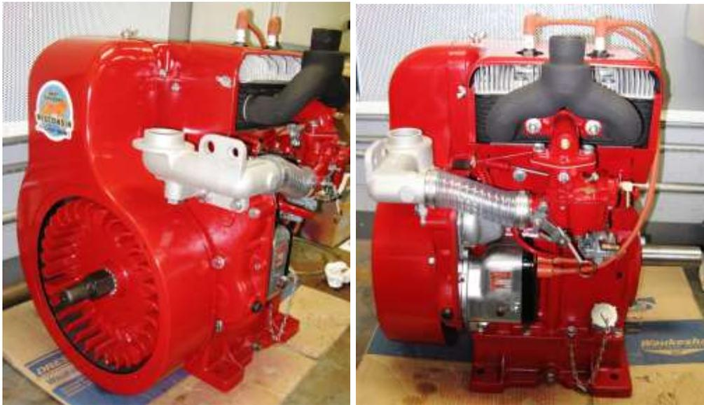
The specification label was not in the best of shape, but some polishing and several coats of clear coat sealant were applied, improving the appearance. It was then screwed into place on the sheet metal shrouding.
