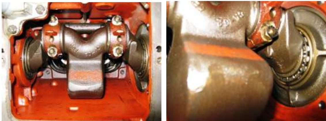
The massive Timken tapered-roller crankshaft main bearings were impressive and attest to the durability that these engines are renowned for.
