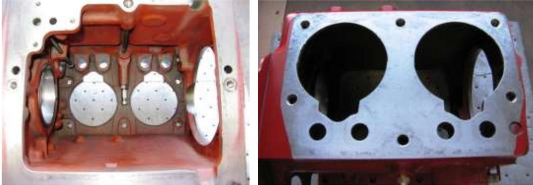
The appropriate surfaces were then masked and the external casting surface was primed and painted. Here the crankcase is shown with the accessory plate plus a few fittings attached.
