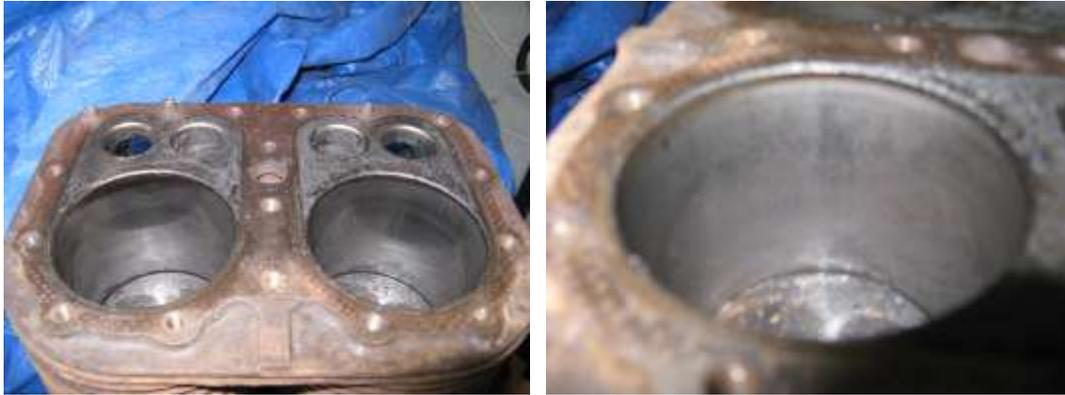
With the poor condition of these top-end parts, it was obvious that a rebore with new pistons, rings, and intake valves had to be done to put this great old engine back to first-class shape.
