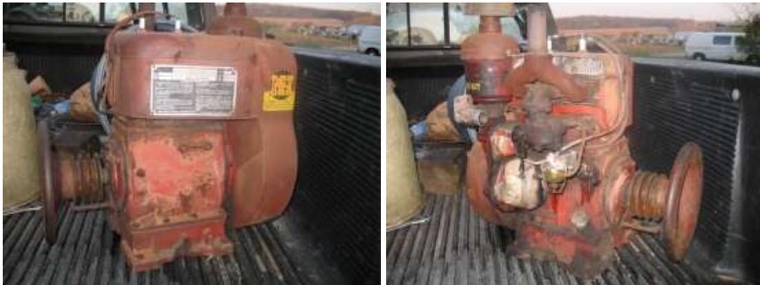
All of the parts seemed to be in place and the crankcase was filled to the proper level with oil. Compression was a bit weak though, and favored one cylinder over the other. The Wico magneto provided a healthy spark, thus a test run was in order.
