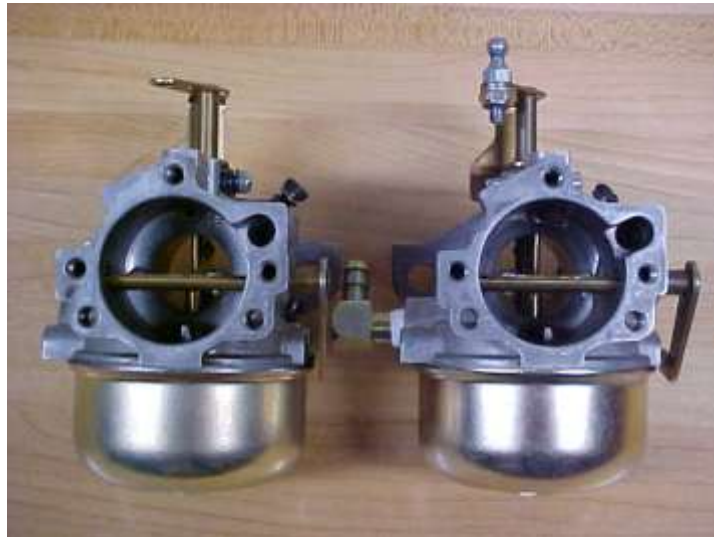
Walbro carburetors – modified one on right
