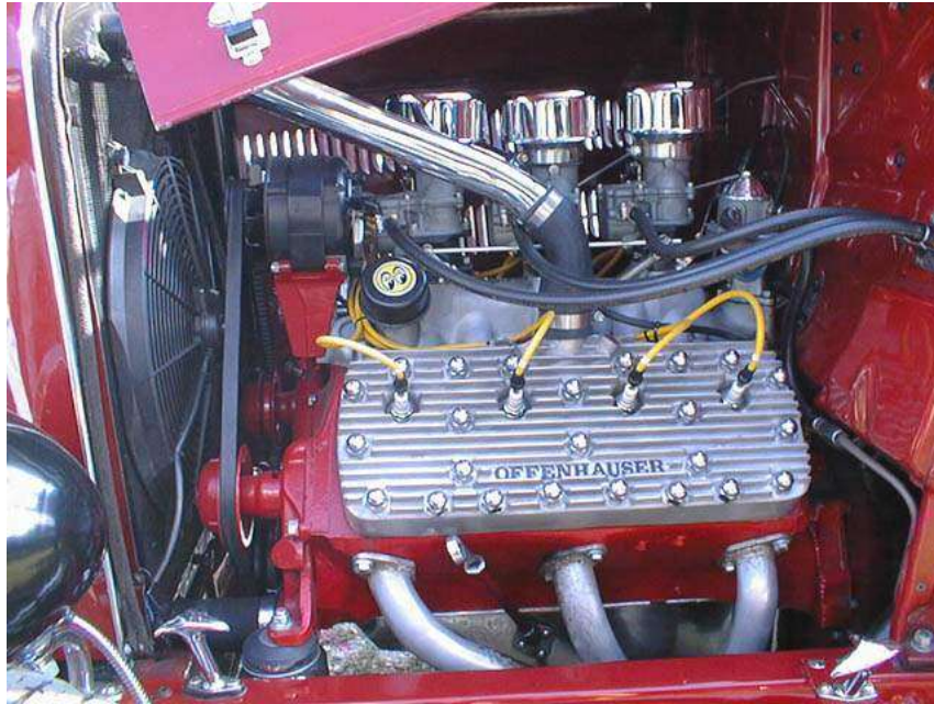
The flathead Ford-Mercury V-8 – A hot rodding classic
