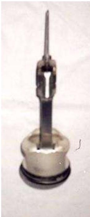
The next important component is the connecting rod. Don Vogt (a highly respected engine builder) turned me on to this one. Kohler made an 18 hp version of the K341, which they called the K361. It was a K341 with overhead valves. But the con rod used in this engine is an Alcoa aluminum FORGING instead of the standard die-cast part. Best of all, this lovely rod fits right into the other engines perfectly. It has the same external dimensions, center distances, and mass as the die-cast rod.
