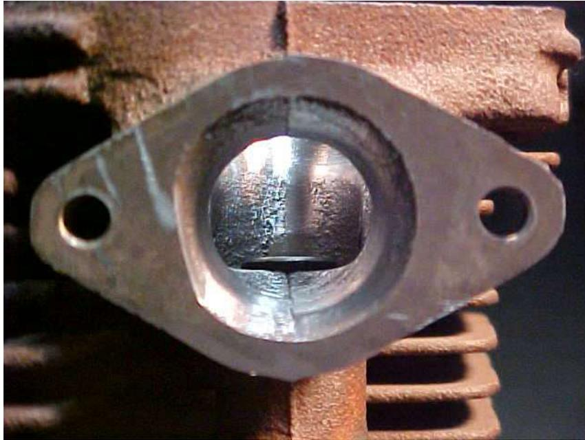
The inside radius of the port is a very important area to blend. Some blocks have rather sharp corners here that need to be blended into a smooth continuous radius
