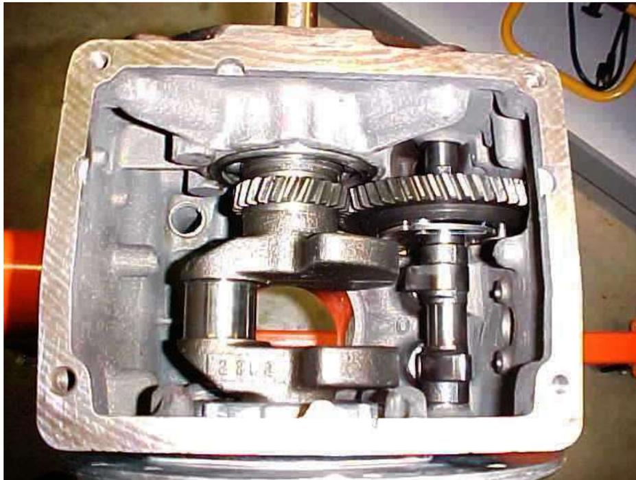
The bearing plate was then fitted using one black and one brown gasket, and bolts torqued to 35 foot pounds. Note new grade 5 bolts fitted. Crank end clearance was checked and found to be .005 in., right in tolerance range.
