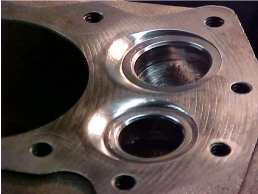
The intake and exhaust ports are next. The stock intake port is formed by a sand core during casting and has the typical rough surface found on cast iron blocks.
