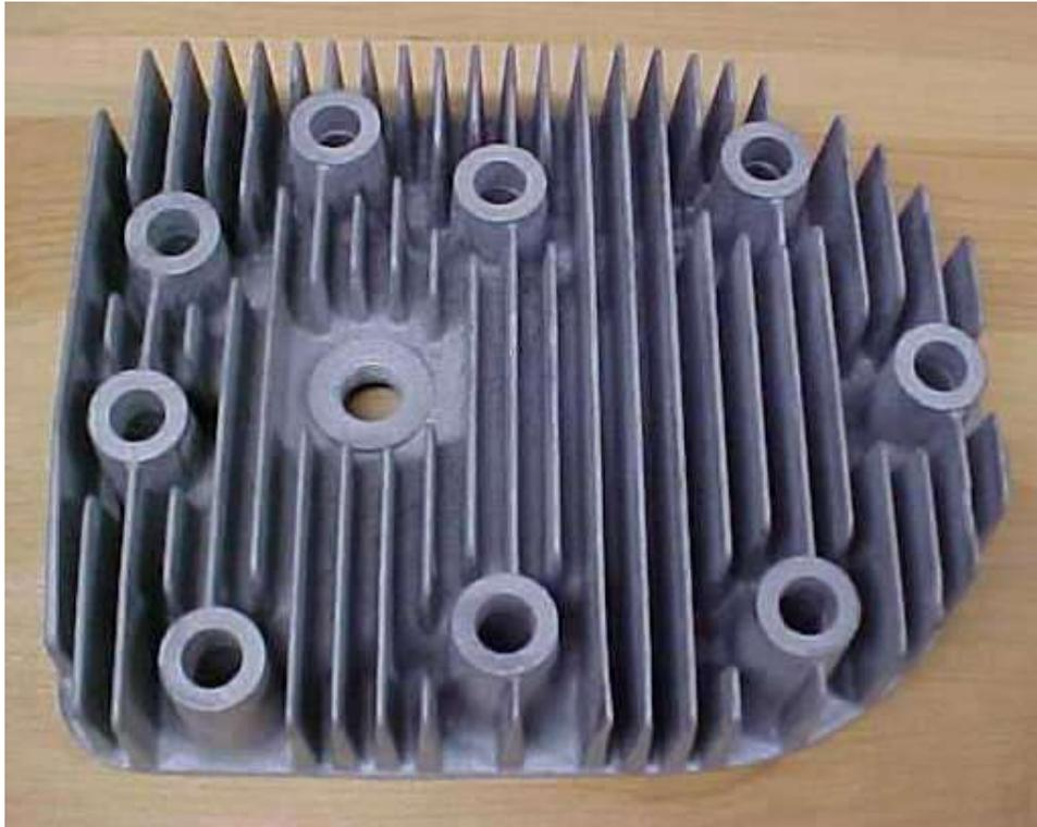
The sealing surface was decked .025 in the mill to raise compression ratio slightly.
